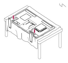
2 Use the screws to secure the stand on the rear side of the product as shown in the diagram.
